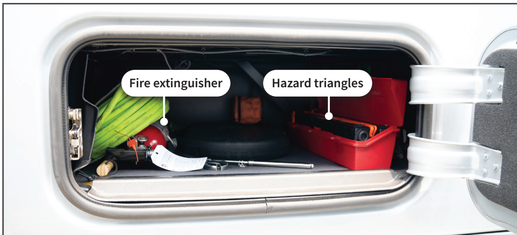
Figure 14. Location of hazard triangles and fire extinguisher
