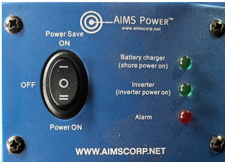
Figure 18. AC power switch (O is OFF)
